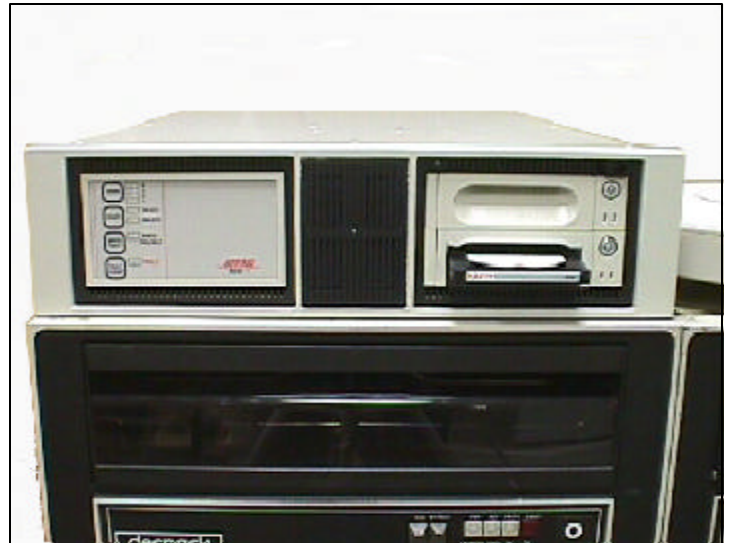
AEM-5C with SCSI drive and removable Jaz cartridge for backup.
