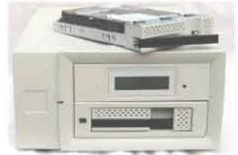
DISK+TAPE Virtual Tape drive -SCSI disk emulating a Tape drive
